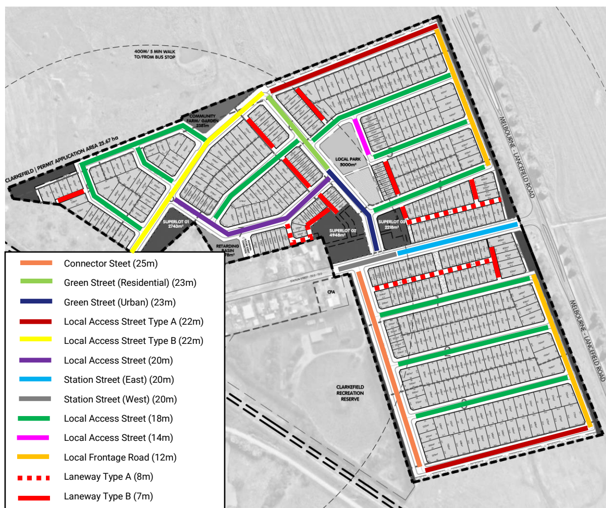
Figure 7: Internal Road Network Plan
